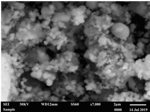
**Fig. 8** Image of scanning electron microscopic observation of synthesized silver nanoparticles
