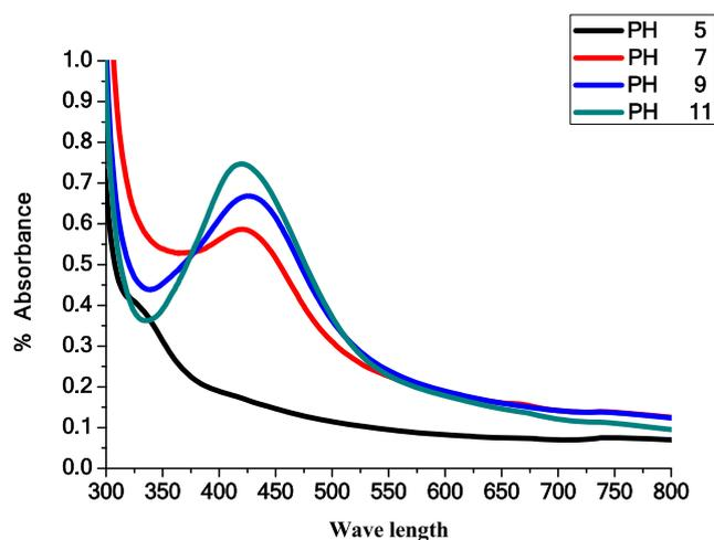
**Fig. 2** UV-vis absorption spectra of Ag NPs synthesized by *Borago officinalis* leaf extract at different PH
