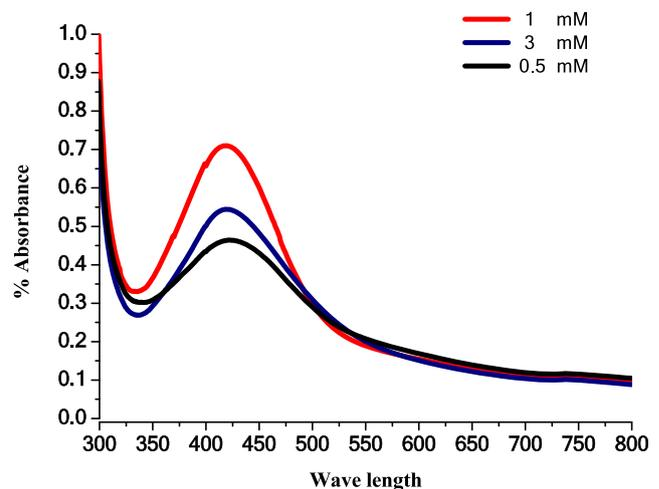
**Fig. 1** UV-vis absorption spectra of Ag NPs synthesized by *Borago officinalis* leaf extract at different  $\text{AgNO}_3$  concentration
